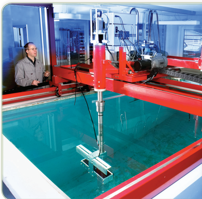
Teledyne RESON Calibration facility
