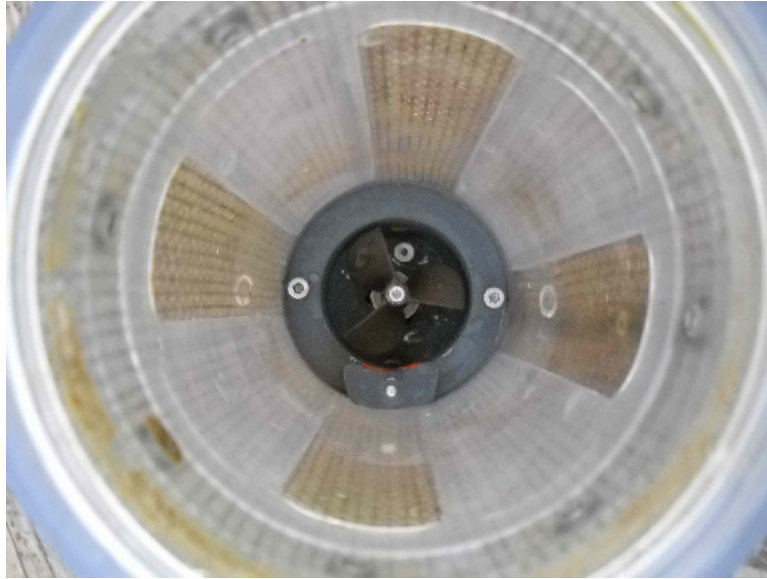
Fig. 2: ProbeGuard sampling chamber after 38 days in Chesapeake Bay
