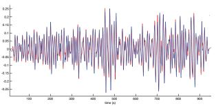
**Heave Performance can be further improved with GPS Aiding.** The whole test was performed in "Vertical Gyro" mode, where only a vertical reference is used to stabilize the attitude. In case of harsh environments, a GPS aiding can be used to improve orientation and heave accuracy, even during long term turns or accelerations, and high amplitude swell conditions.
